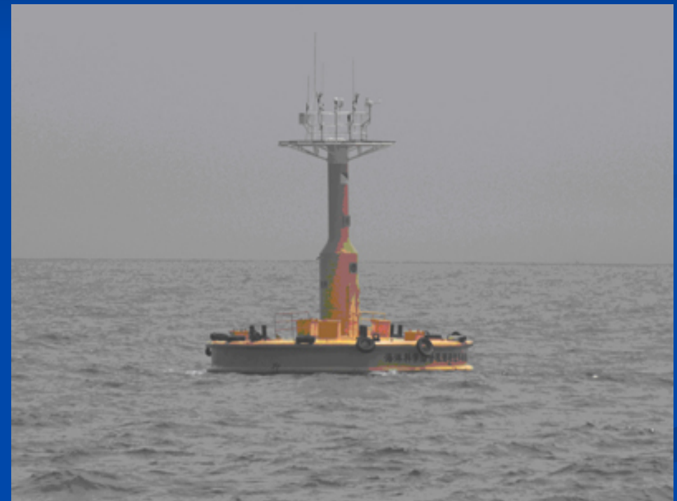
The marine observation buoy in east of Shengshan (嵵山)
